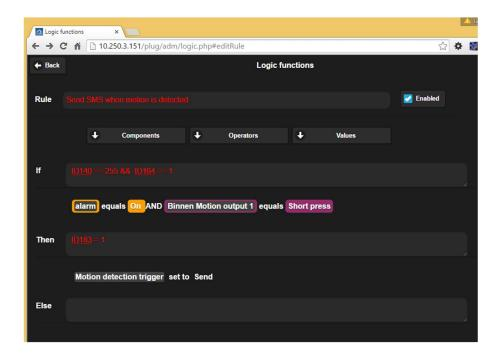
The rule will be triggered when the alarm is active (ID140 == 255) and the motion sensor is triggered (ID164 == 1)
